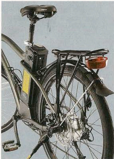
The pannier rack, lights, mudguards and kickstand make this a utilitarian machine
